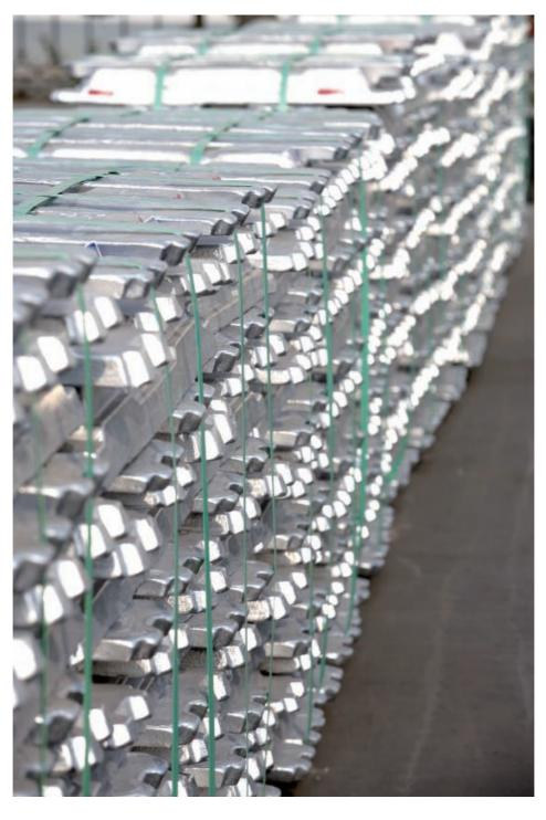
Sales of aluminum alloy ingots accounted for approximately 43.5%, 37.5%, 15.1% and 23.4% of our revenue generated from aluminum products for 2008, 2009, 2010 and the three months ended March 31, 2011, respectively. Molten aluminum alloy is processed into aluminum alloy ingots through molding, casting and cooling. Our aluminum alloy ingots are produced by using self-manufactured molten aluminum alloy.
